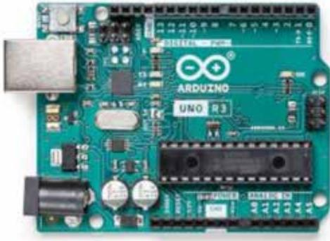
Figure 2 (a): Arduino UNO Board
